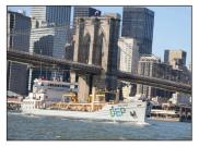
NYC for the first time-with a capacity of 150,000 cubic feet-approximately 50% more than our other two self-propelled sludge boats.
