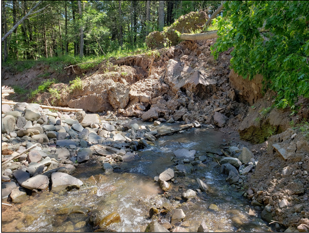
Figure 2. Looking downstream at the primary failure and fine sediment sources.
