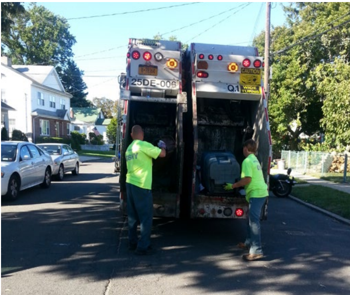
Dual-bin trucks have a split hopper so that refuse can be collected on one side, organics on the other.
