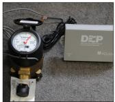
Now: A ¾ inch Elster InVision Water Meter, Encoder Type, measures in cubic feet. A radio frequency (RF), Meter Transmission Unit (MTU) by Aclara Technologies is attached as the latest style of Automatic Meter Reading (AMR) equipment.
