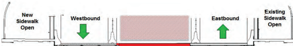
Stage 2 - Center Roadway - 12 Months. The Center Roadway will be Closed. All Traffic Shifts to One Eastbound and One Westbound Lane in Each Direction.
