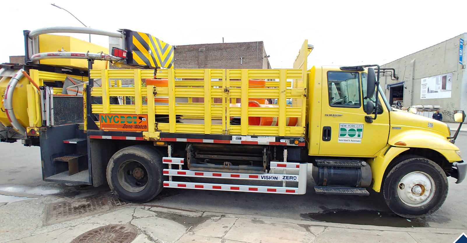
A side guard installed on a Department of Transportation truck.
