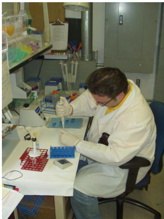
Figure 3.12 DEP Pathogen Laboratory staff micropipetting a concentrated water sample for microscopic analysis of Giardia and Cryptosporidium .
