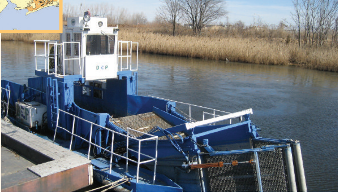
Floatables skimmer vessel in Hendrix Creek
