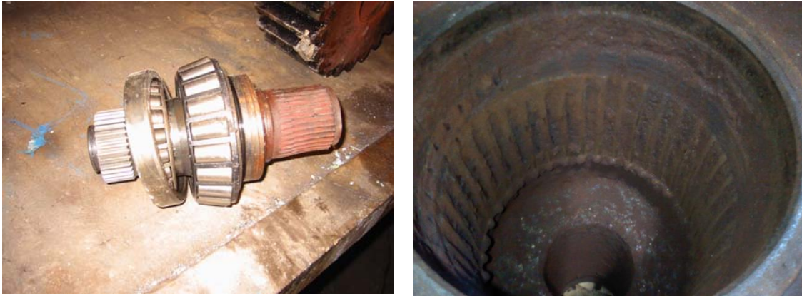
Figure C.6.4: Worn Pinion and Pinion Spine
