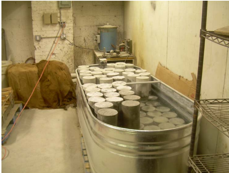
Figure 1: Improper Cylinder Curing Procedures, Some Cylinders Partially Immersed
