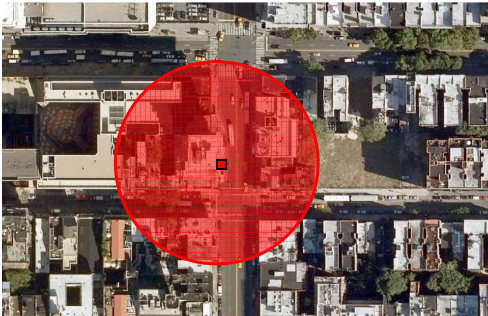
Figure C.1.2: Impact Zone of a Tower Crane Collapse.
