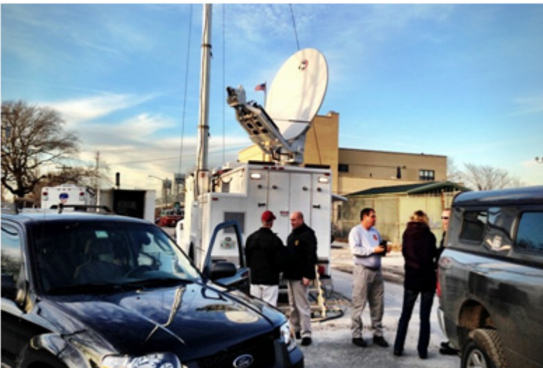
DoITT's cell-on-wheels tower – one of many deployed in the impacted zones – beamed out cell service through the vertical mast.
