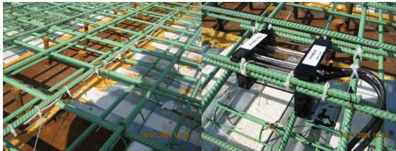
The Corrosion Monitoring Probe Sensor Measures the Electrical Potential Between the Rebar and the Electrode. The Corrosion Penetration Monitoring Probe Sensor Measures Corrosion Caused by Chlorine Containing Moisture.
