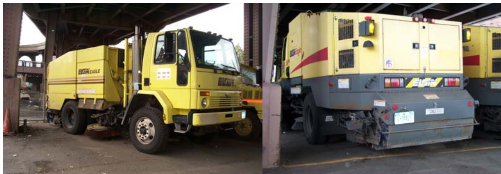
Mechanical Sweeper – Side and Rear Views. (Credit: Peter Basich)
