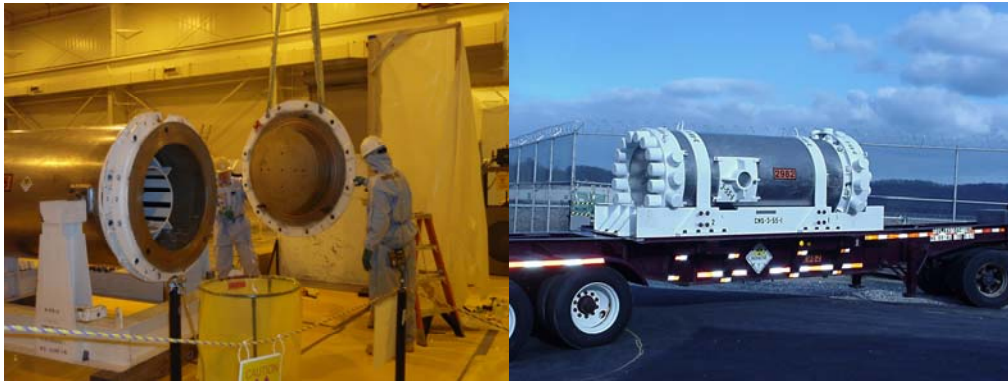
In February 2009, a Permit Was Issued for the Move of the Beam Plug of a High Flux Beam Reactor From Brookhaven National Laboratory. The Plug Was Loaded Into a Steel-Supported, Lead Lined Shipping Cask. Although the Metal is Radioactive, the Radiation Cannot be Dispersed. The Driver Was Federally Certified, Accompanied by Armed Escorts, and Only Traveled at Night.
