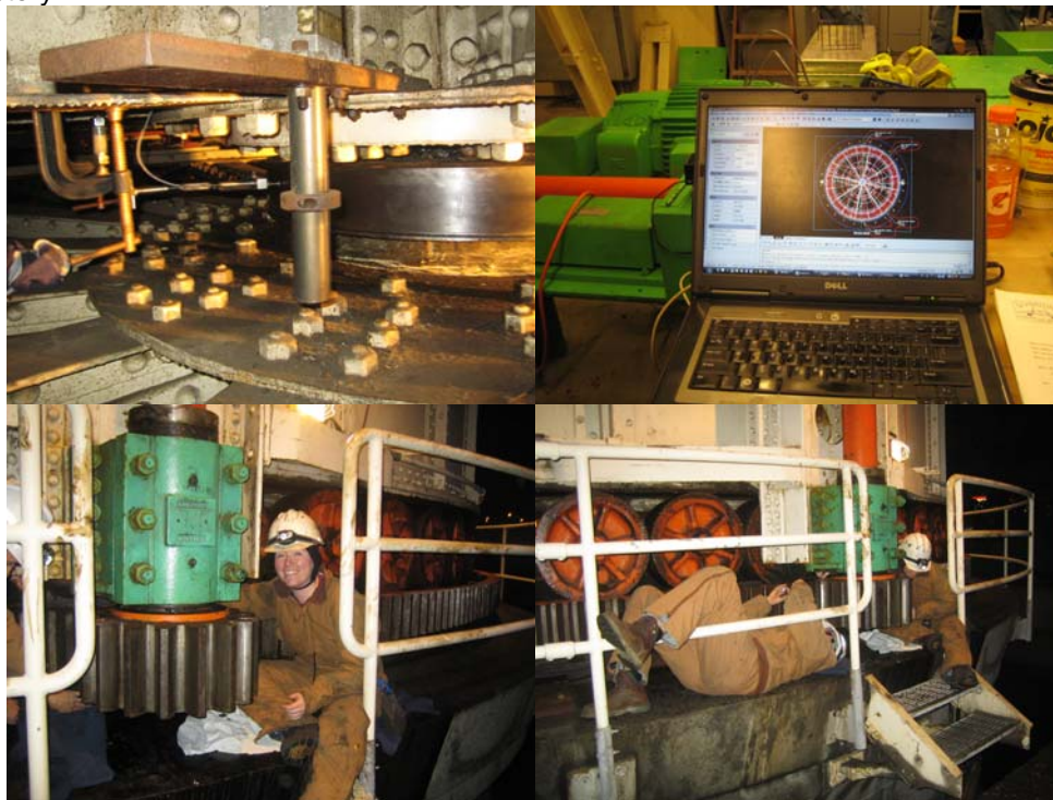
Macombs Dam in October 2009. Displacement Sensor Recording the Position of the Center of the Bridge During a Bridge Opening. Sensor Recording Program. Measuring Tooth Backlash for the Concentricity Test. (Credit: Vera Ovetskaya)
