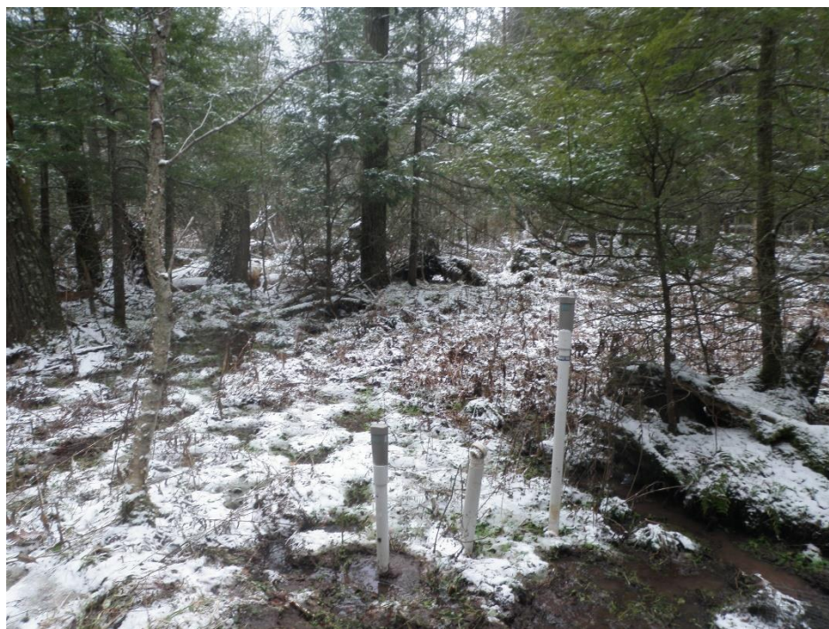
Figure 4.17 New water level logger installed between two older loggers in a reference wetland site in the Pepacton Reservoir basin.
