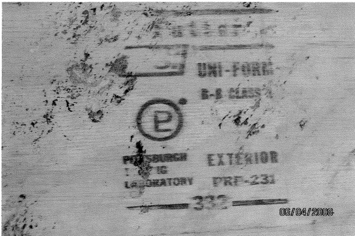
Photo 16 - 4'x8' plywood sheet with a Futter Lumber Company grade stamp.
