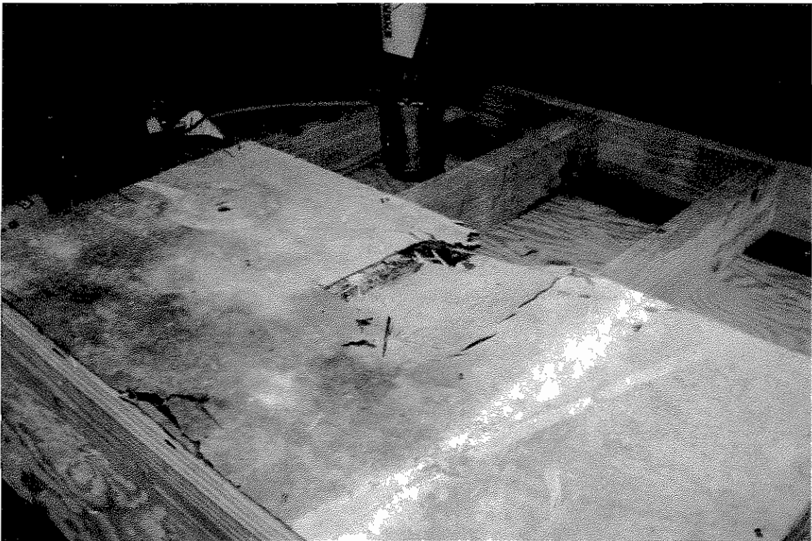
Photo 26 - Punch through failure of test specimen TP9-A.
