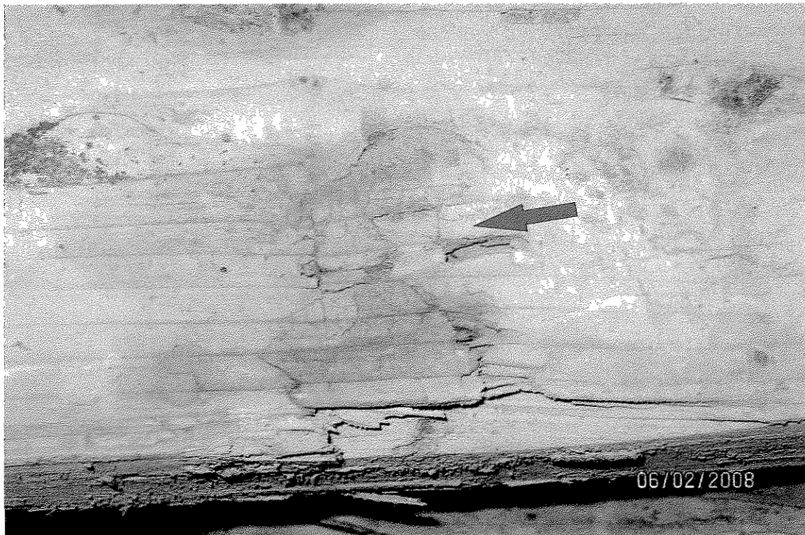
Photo 8 - Visible wood decay growth on 3x4 lumber specimen marked DOB #TB40291.
