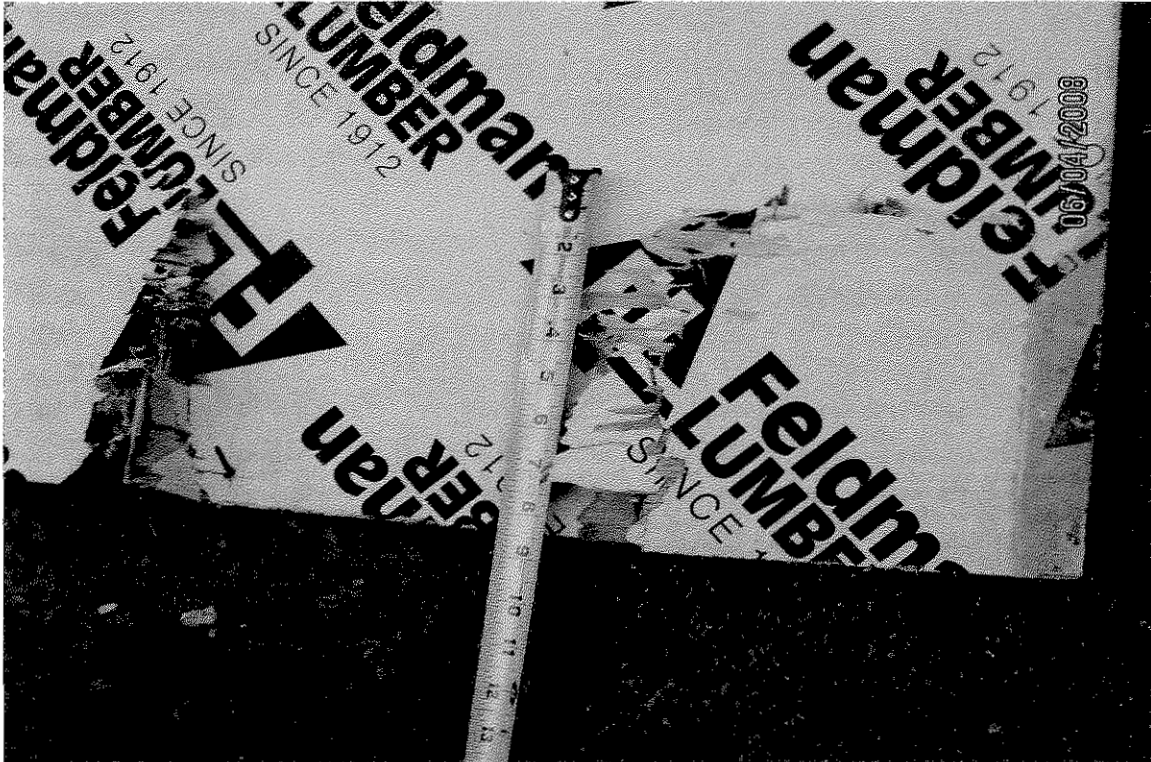
Photo 19 - Failure pattern consistent with a base plate punch through failure in panel DOB #PW41003.
