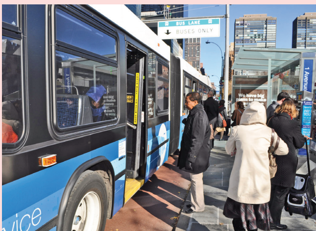
M15 SBS allows riders to board the bus from all three doors, thanks to fare pre-payment at on-street fare machines.
