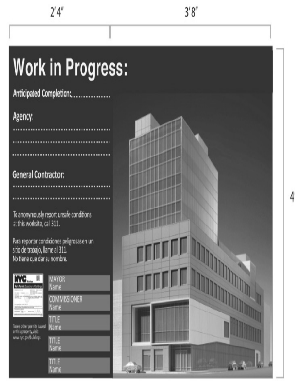
FIGURE 2 FENCE PROJECT INFORMATION PANEL LAYOUT
