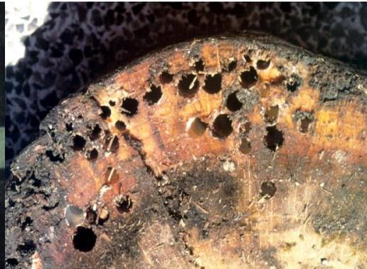
Teredo Damage (holes up to ¼" diameter)
