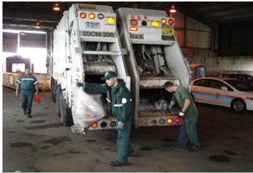
Sanitation workers unload collections, which are separated in a dual bin truck. DSNY supervisors and staff from DSNY's Operations Management Division ensured tracking of origins of all collections.
