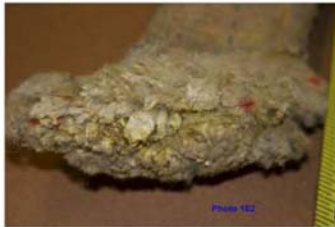
Figure 7. Fracture surface of sling piece 4A.
