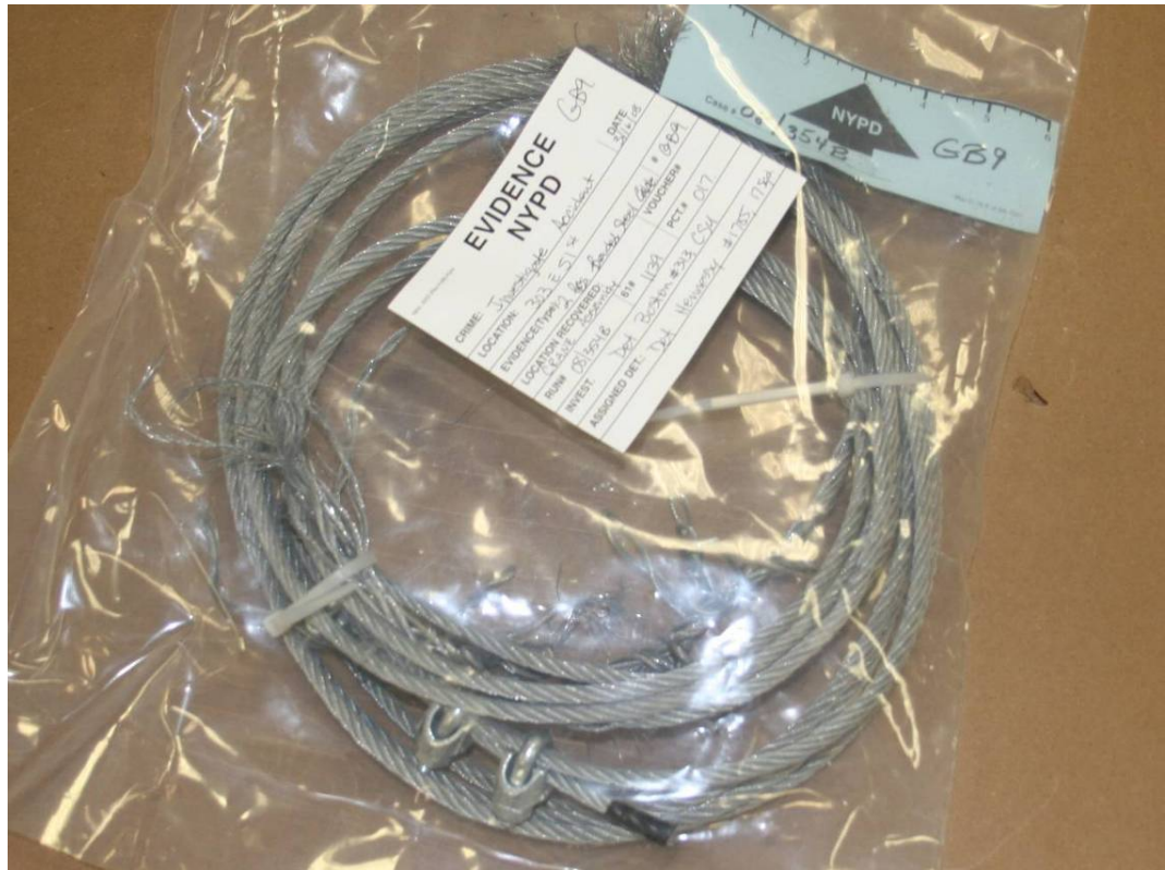
Photograph 3.2 - OSHA retained evidence from NYPD GB9. Note the two clips only, with the saddle on the dead end of the wire rope. Photo by Arup.
