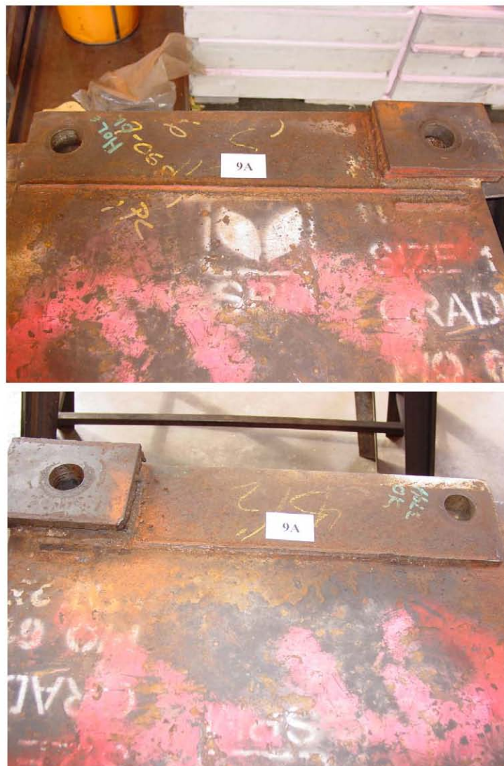
Figure 11 General Views of the Weld Fracture on Base Plate 9A.
