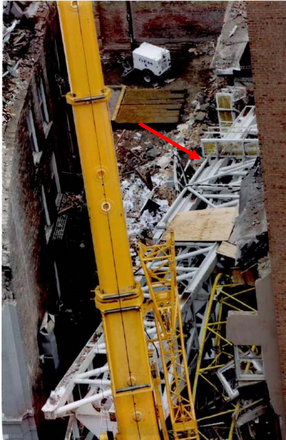
Photograph 1.6 – Photograph showing the external climbing frame attached to top of tower at the time of the collapse (source: Photos by the New York Police Department, Pictures 117-178, page 3 of 62).
