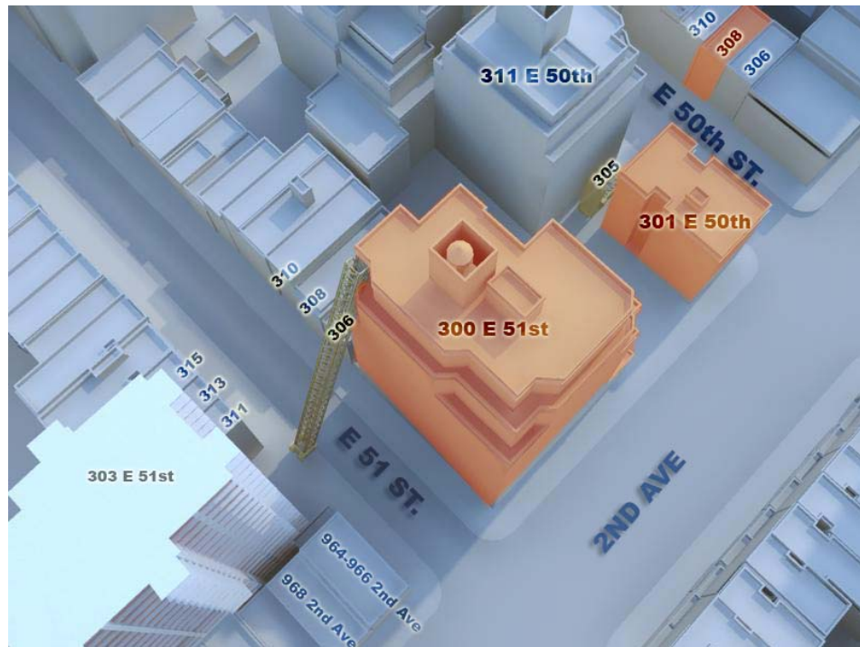
Figure 1.12 - Representation of the tower crane after collapse. Reference Photograph 1.6 with regard to the position of the crane within 305 E 50 th St. Prepared by Arup.
