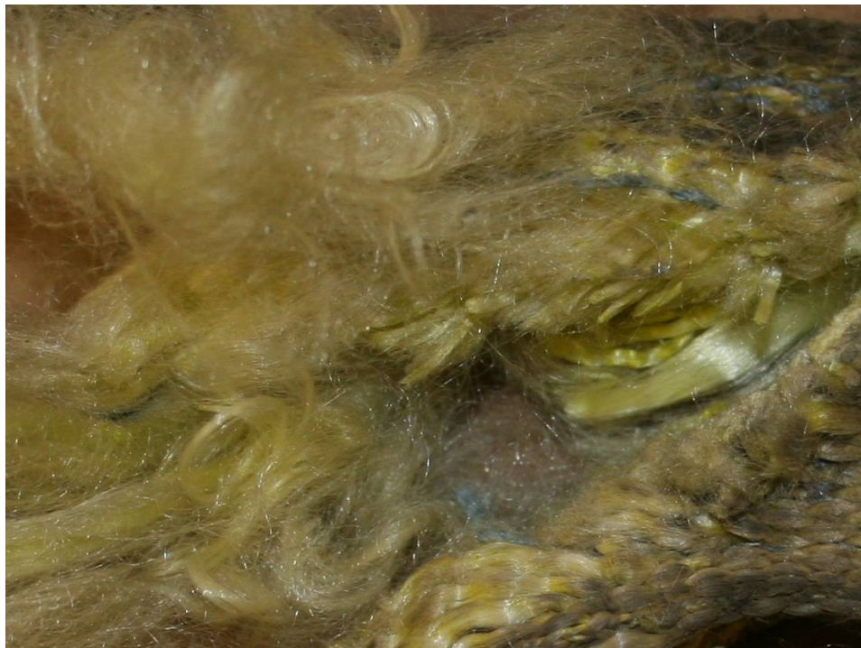
Photograph 3.9 - OSHA evidence item 1. Polyester web sling removed from the collapse site. This was taken from the southwest corner of the 9th floor collar. Note the varying degrees of fading of the webbing coinciding with the relative degree of potential exposure to ultraviolet rays. Magnification is approximately 2.5x. Photo by Arup.
