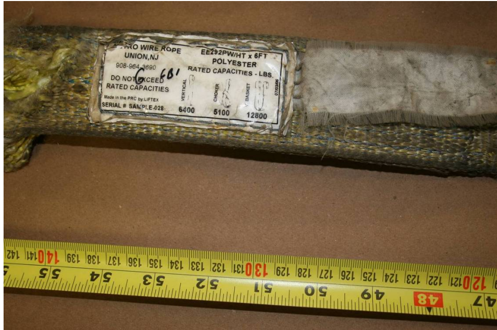
Photograph 3.8 - OSHA evidence item 1. Polyester web sling removed from the collapse site. Note the faded label. This was taken from the southwest corner of the 9th floor collar. It was attached to the lifting point via a chain fall. Photo by Arup.
