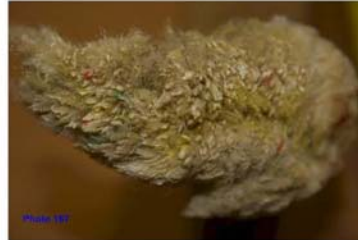
Figure 8. Fracture surface of sling piece 7A.
