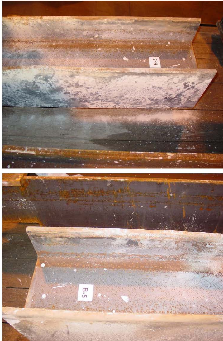
Figure 17 General Views of Weld Fracture on Tie Beam B5.
