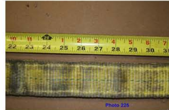
Figure 11. Evidence of high stress along a line on sling piece 13.
