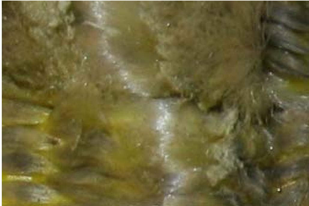
Photograph 3.17 - Close-up of both cut and melted fibers for OSHA item no. 2. Magnification approximately 9x.. Photo by Arup.
