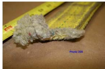
Figure 10. Fracture surface of sling piece 12.
