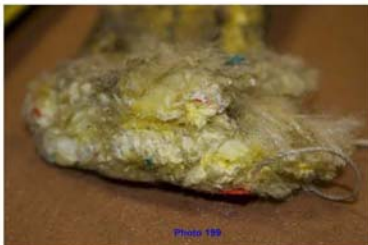
Figure 9. Fracture surface of sling piece 11.
