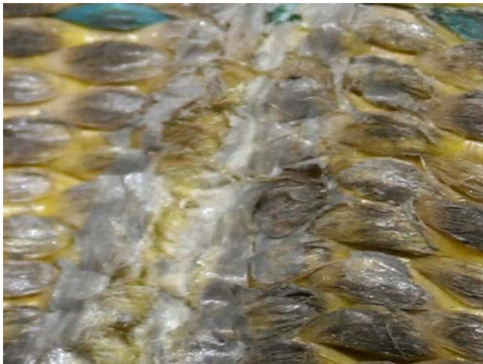
Photograph 3.11 - OSHA evidence item 1. Polyester web sling removed from the collapse site. This was taken from the southwest corner of the 9th floor collar. Note both the melted and cut fibers within the melted region. Magnification is approximately 10x. Photo by Arup.
