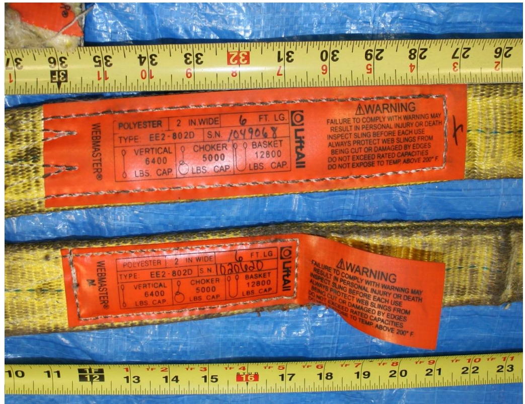
Photograph 8.4 - Warning labels on slings recovered from the collapsed tower crane clearly require inspection before use and use of protection at all edges. Photo by Arup.
