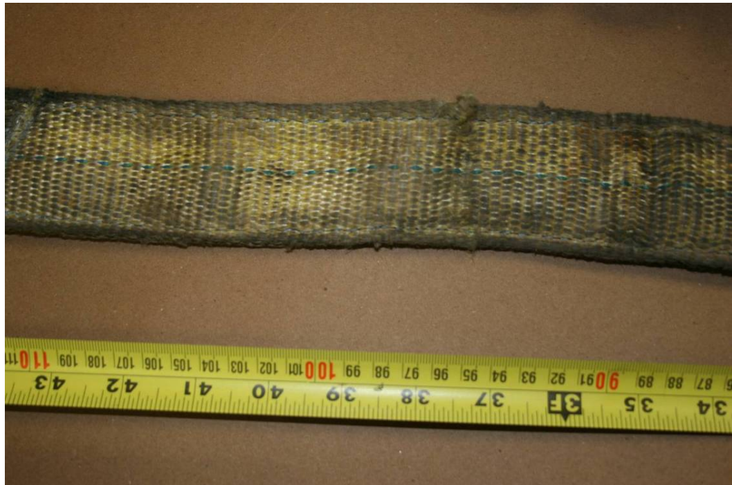
Photograph 3.18 - Liftex polyester web sling (OSHA item no. 1). Damage can be seen along the edges, as well as wear within the width of the sling, at uneven intervals, unlike the other polyester web slings where damage occurs at approximately 12 inch intervals. Photo by Arup.
