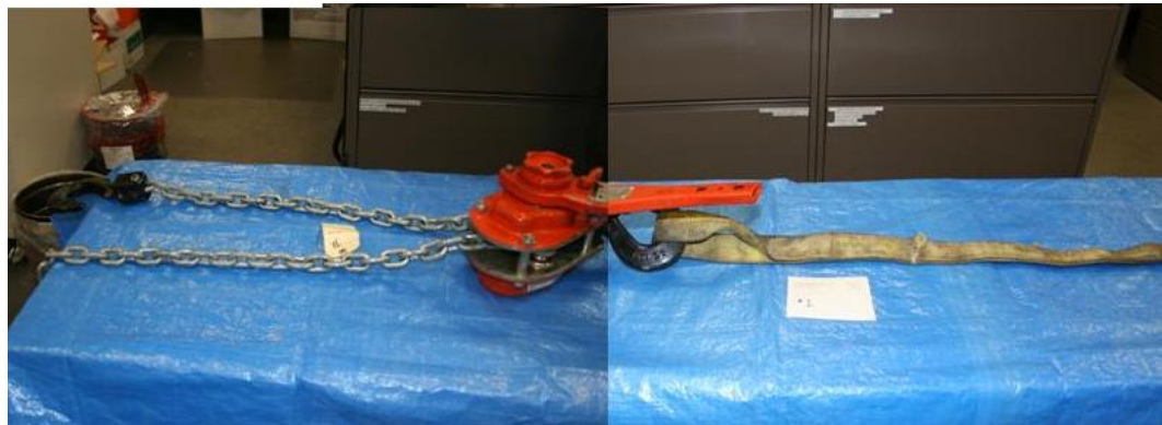
Photograph 1.8 – Chain-fall and polyester sling assembly recovered from collapse site by Arup.
