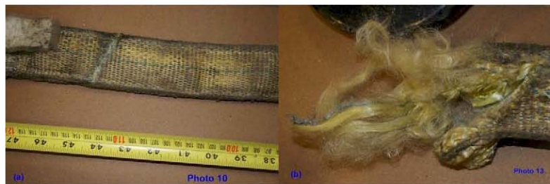
Figure 3. (a) Sign of stress on sling piece 1A, (b) Fracture surface of sling piece 1A
