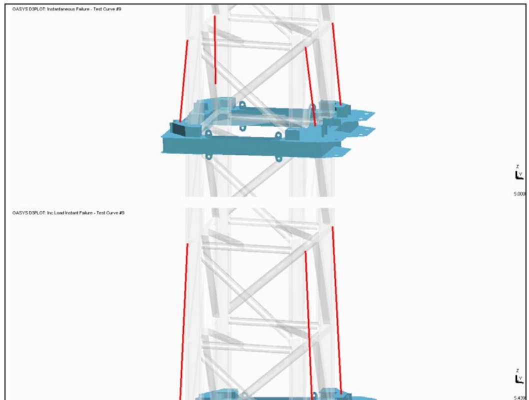
Figure 8.22 - Deformed Mesh at end of Curve #9 Analyses (uniform initial sling load top –non uniform initial sling load bottom). Prepared by Arup.
