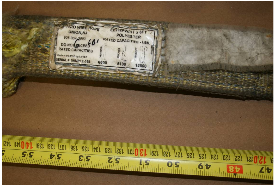
Photograph 8.6 - Metro/Liftex sling recovered from tower crane. Not the faded label and faded appearance of the sling exterior. Photo by Arup.
