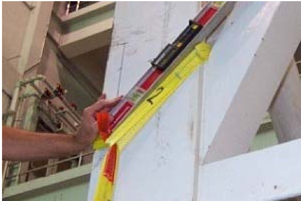
Photograph 3.19 - ATLSS test setup prior to testing. Note that, as installed around the tower leg in the V-groove formed between the diagonal and the leg, the sling will necessarily be constricted, bunched and pinched by the load. Photo provided by OSHA.
