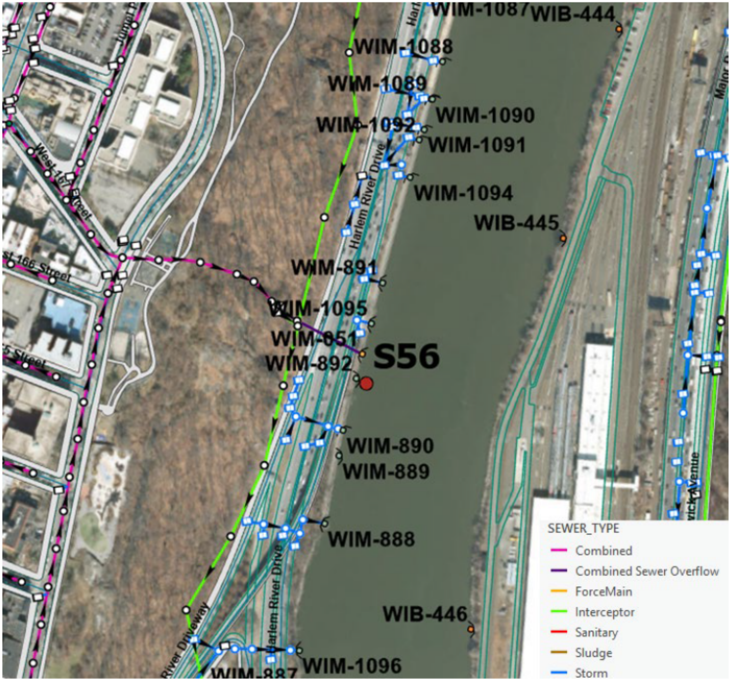
S56 and the CSO and MS4 outfalls in the area
