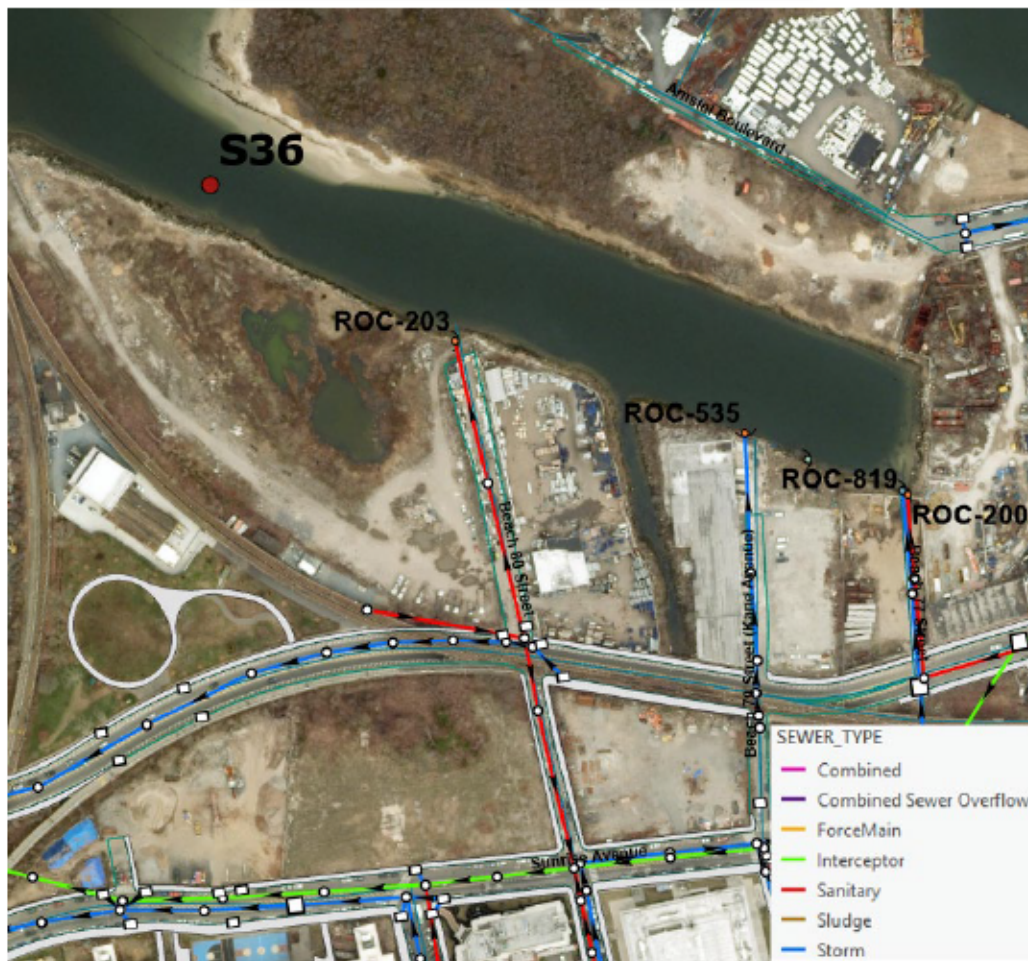
S36 and the sewers in the sentinel station area. The sewer map requires changing.
