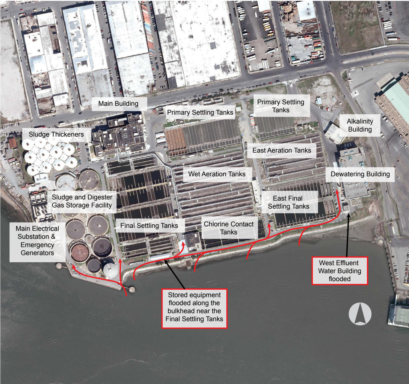
Flood pathways and areas flooded during Hurricane Sandy are highlighted in red.
