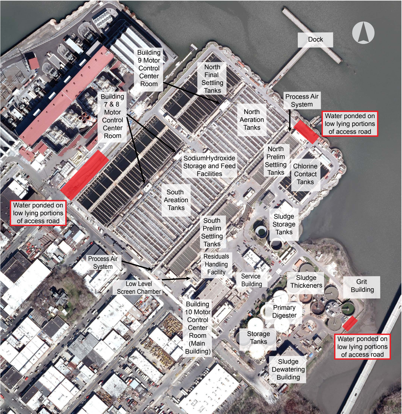
Flood pathways and areas flooded during Hurricane Sandy are highlighted in red.
