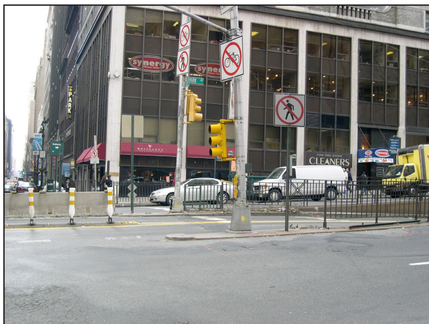
Pedestrian signage, iron pedestrian fences and other roadway improvements discourage pedestrians to cross at this location and provide for safer vehicular movements
