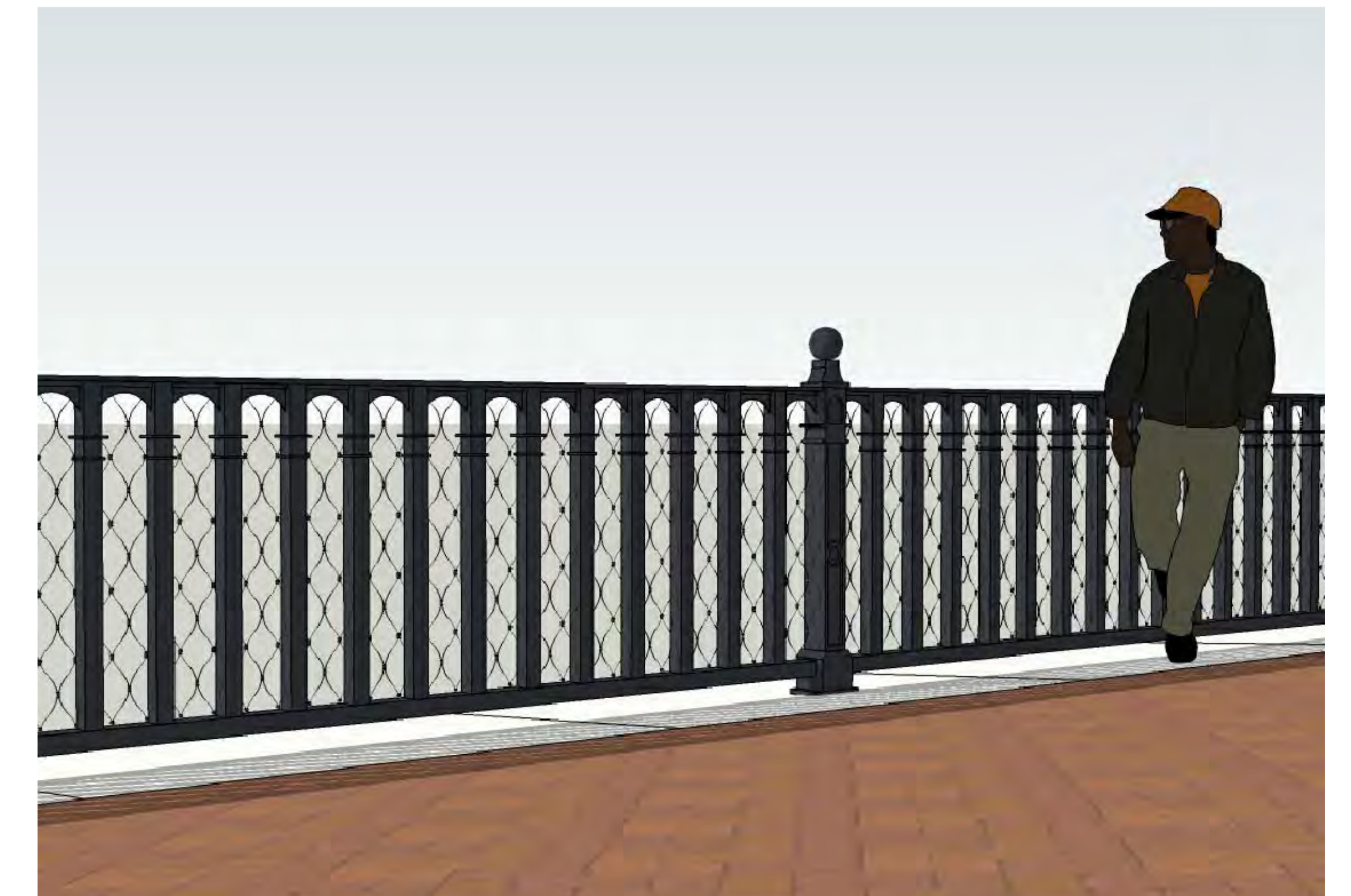
6 STAINLESS STEEL CABLE MESH DETAIL VIEW SCALE: 1/2" = 1'-0"
