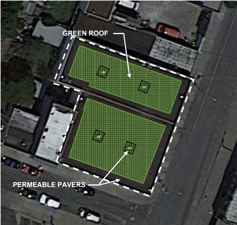
SITE SCHEMATIC with STORMWATER CONTROL MEASURE (SCM)
