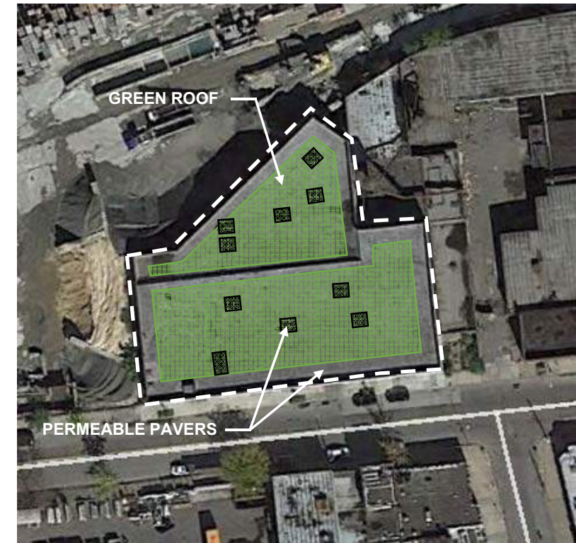
SITE SCHEMATIC with STORMWATER CONTROL MEASURE (SCM)
