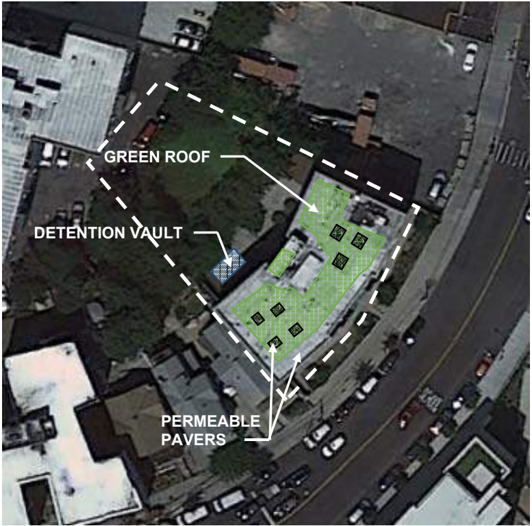
SITE SCHEMATIC with STORMWATER CONTROL MEASURE (SCM)
