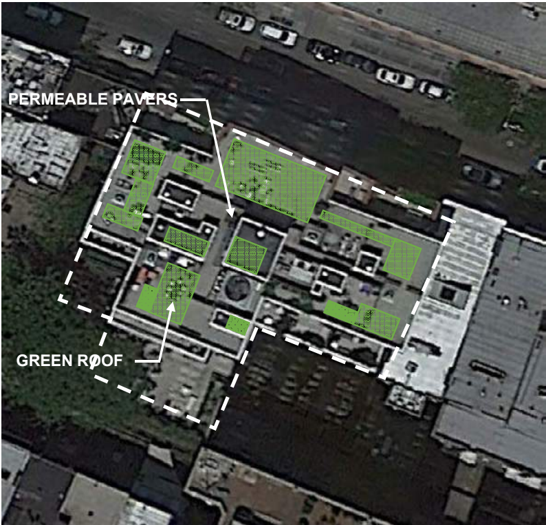
SITE SCHEMATIC with STORMWATER CONTROL MEASURE (SCM)
