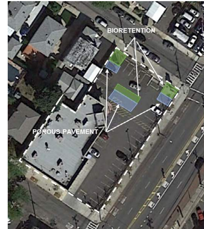
Figure 6-5: Example Bioretention Practice with Underdrain and Permeable Pavement (Commercial and/or Mixed-Use Category B – Subsurface Constrained, Space Unconstrained)
