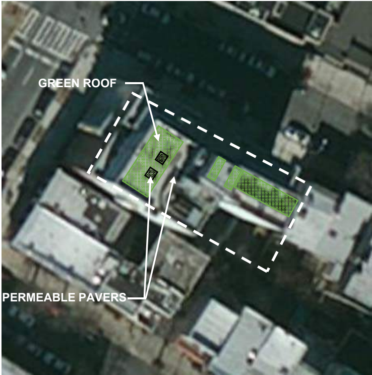
SITE SCHEMATIC with STORMWATER CONTROL MEASURE (SCM)
