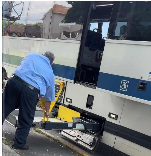
Figure 3: Wheelchair Lift Could Not Be Raised because Driver Performed Steps Out of Sequence
