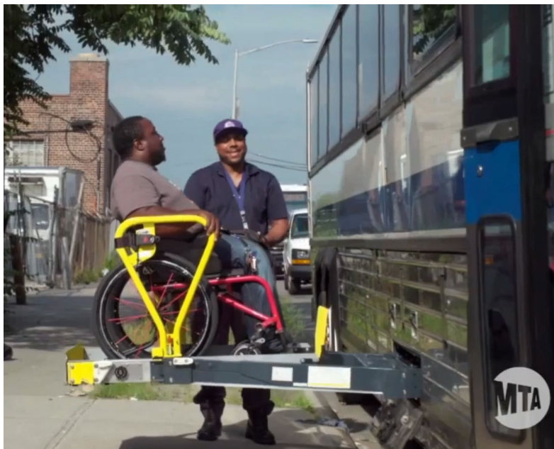
Figure 2: MTA Express Bus with External Wheelchair Lift
