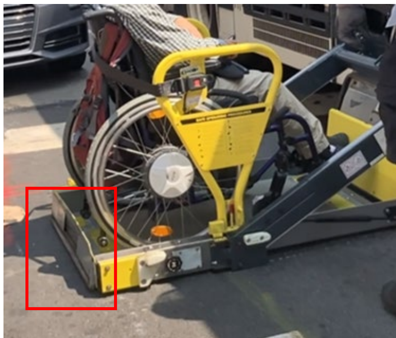
Figure 5: Wheelchair User Incorrectly Positioned on Lift Platform
