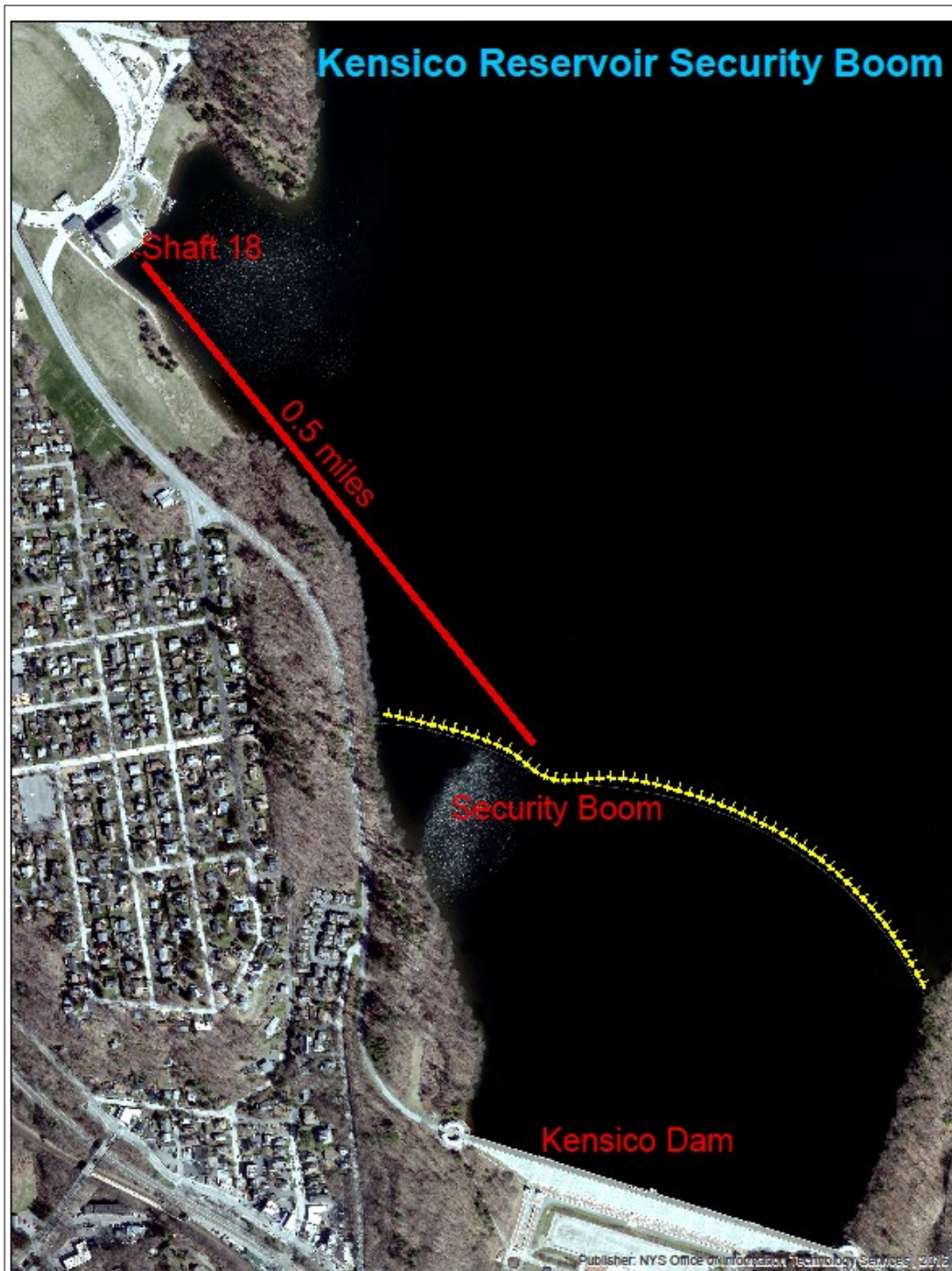
Figure 3.8. Distance from the Kensico Reservoir Dam security boom to Shaft 18.
