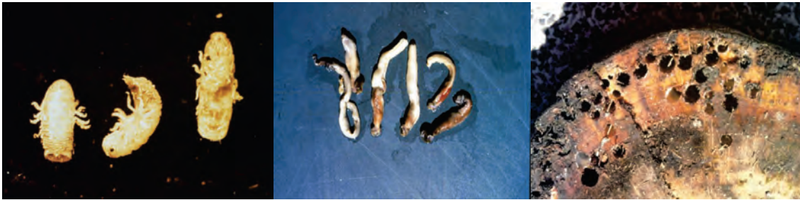
Marine Borer – Limnoria Species (the Common “Gribble,” a Genus of Crustacea Borers). Marine Borer – Teredo Species (a Genus of Molluscan Borers, Commonly Called the “Shipworm”). Teredo Damage (Holes up to ¼” Diameter).
