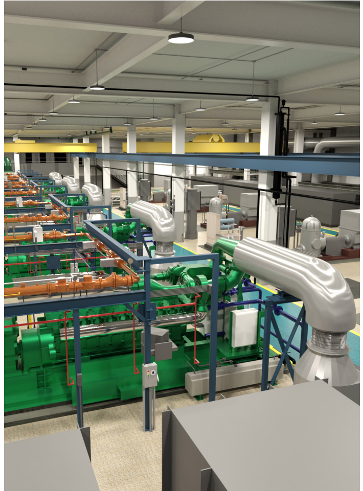
Figure 1: Rendering of cleaner-burning co-generation engines at West Harlem's North River Wastewater Resource Recover Facility
