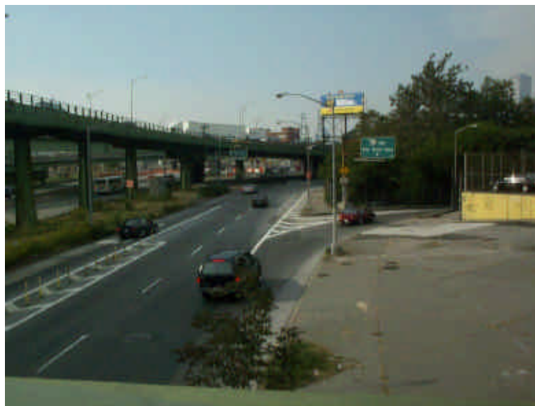
Figure 7.3. New striping and treatment implemented in 2001 restricts weaving on Hamilton Avenue at the BQE.
