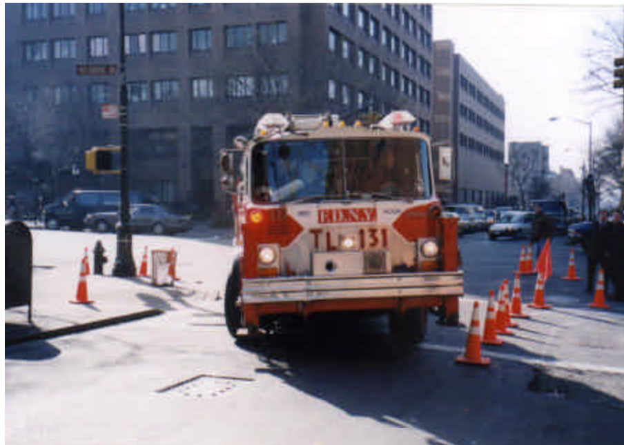
Figure 7.1 Testing the Hicks Street neckdown for FDNY turning radius
