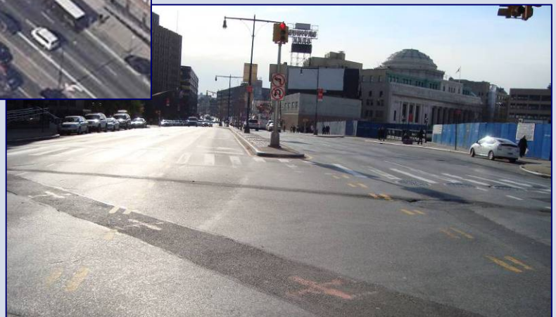
Flatbush Avenue at Willoughby Street facing south – long crossing distance with no protection at median from turning vehicles
