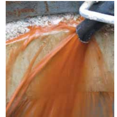
Biofilm and precipitated iron pumped from well
