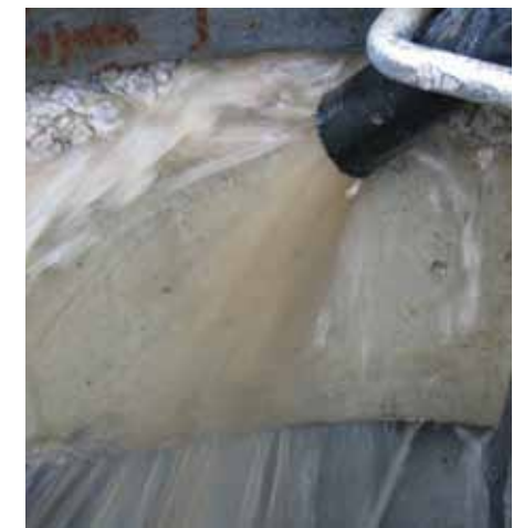
Clear ground water after impulse generation
