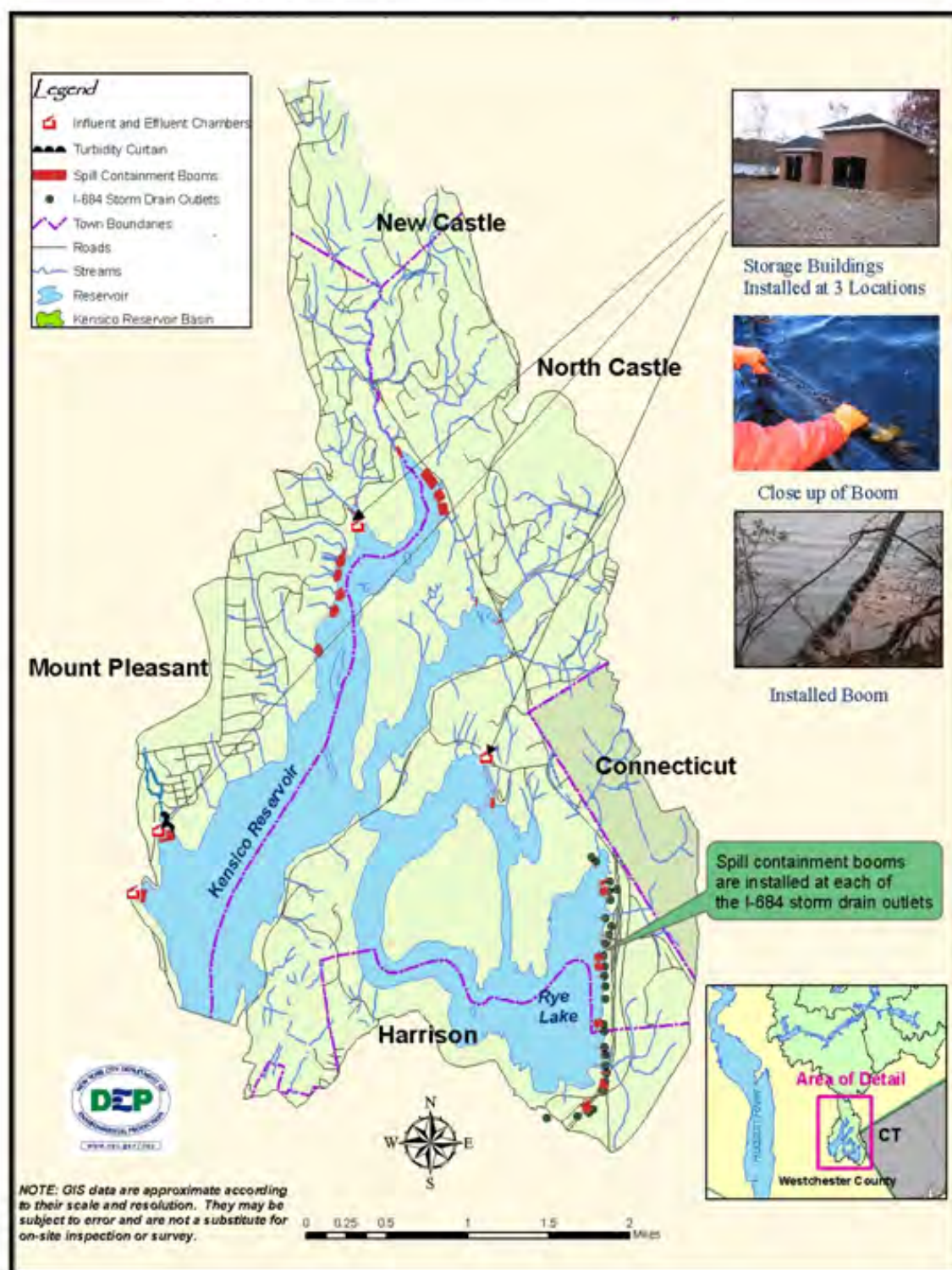
Figure 1.3 Spill containment facilities in Kensico Reservoir.
