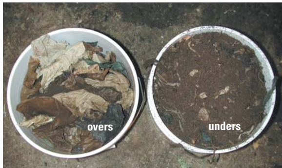
Photo 1-13: Samples taken from the NYC two-inch unders (right) and overs (left) piles
