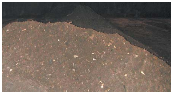
Photo 1-12: Two-inch trommel screen "unders"
