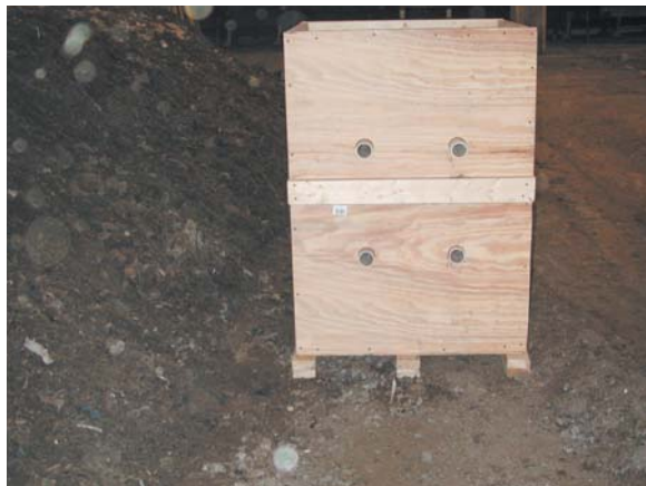
Photo 1-16: Cubic-yard sample shipped to lab for additional curing and testing The sample cured at the lab for an additional 21 weeks. At different points during this period, lab staff removed samples for analysis.
