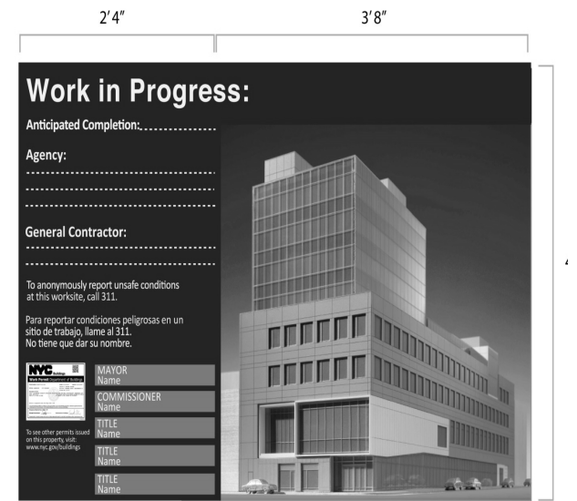
FIGURE 2 FENCE PROJECT INFORMATION PANEL LAYOUT
