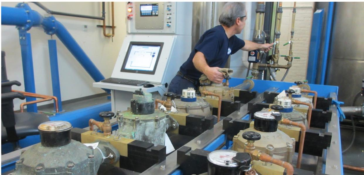
At our Meter Test Facility, DEP employees carry out critical testing and upkeep to monitor the accuracy and coordinate necessary repairs of our water meters.
