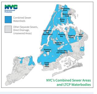
Tanks CSO retention tanks are large facilities that capture CSO discharge during a wet weather event and pump it back to a wastewater treatment facility after the storm when there is capacity in the sewer system. NYC has four existing CSO tanks: Alley Creek, Flushing Creek, Jamaica Bay tributaries: Paerdegat Basin, Spring Creek.
