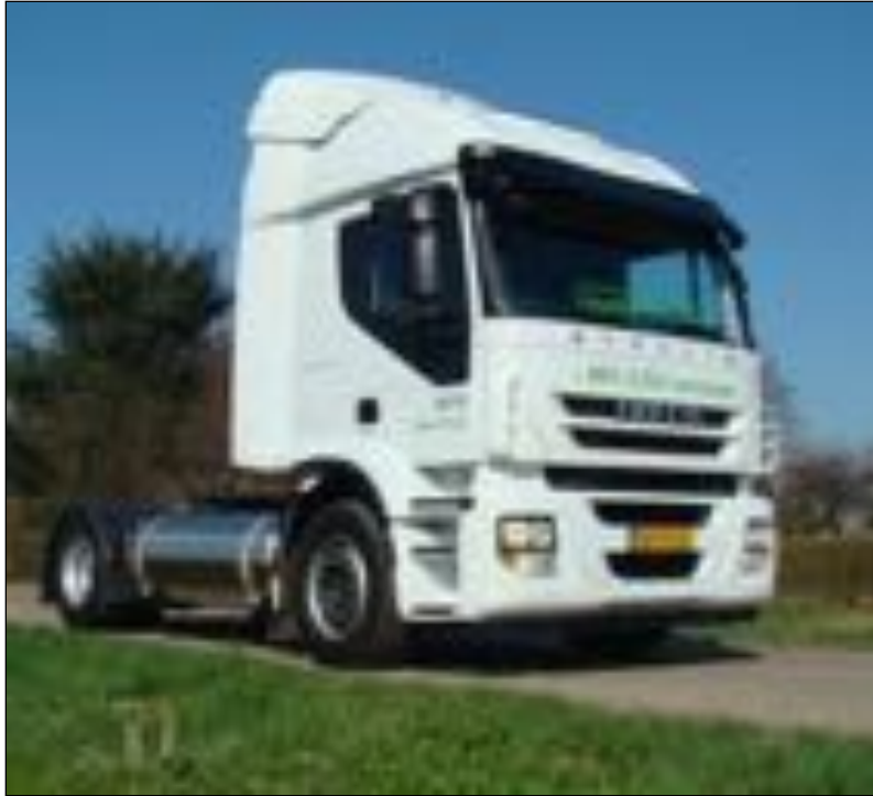
Figure A.145: Iveco Stralis - Compressed Natural Gas (CNG) Engine (Goevaers, 2011)
