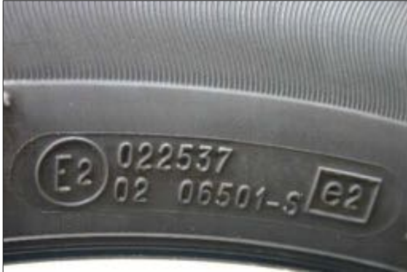
Figure A.148: Tire Showing "S-marking" (BANDVULC Group, 2009)
