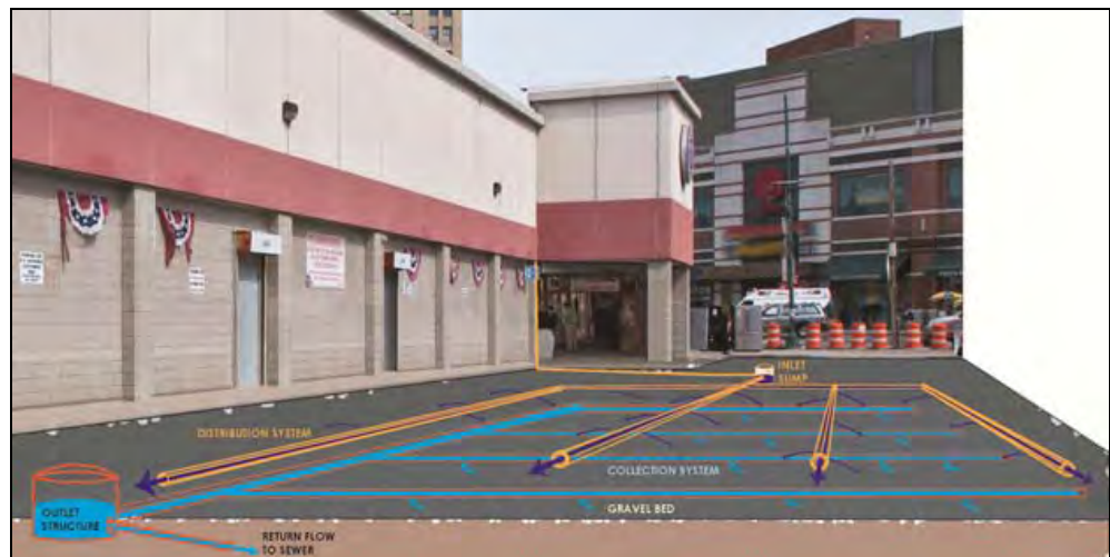
Sample diagram in draft guidelines illustrating potential subsurface configuration of a gravel bed under a parking lot
