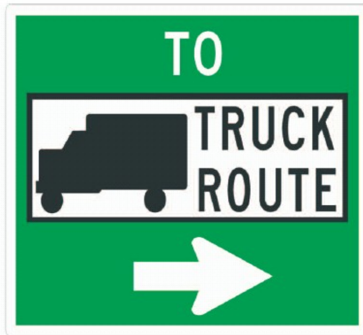
Figure 39 Truck Route Trailblazer Sign NYCDOT Sign Panel Layout
