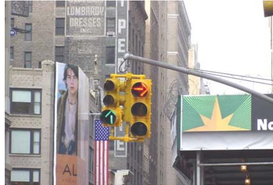
Figure 7. Split Phasing Signal
