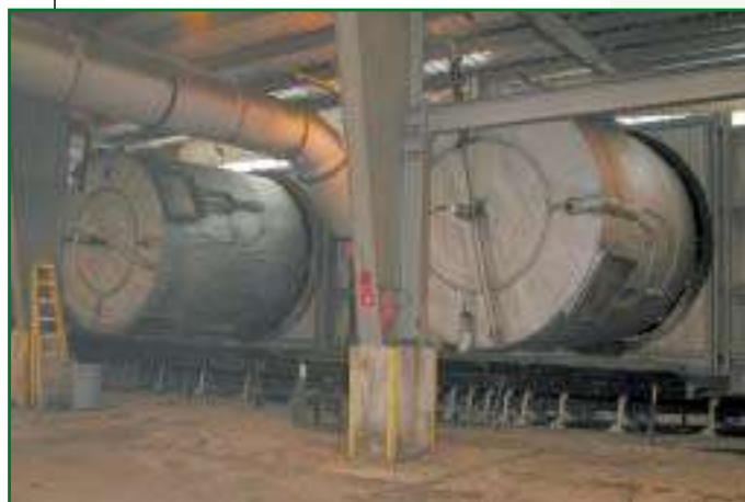
A view inside the building where material is discharged from the composting drum. The conveyor belt under the drum moves the material to a two-inch trommel screen.
