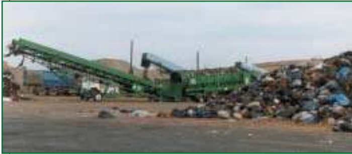
At compost sites, collected leaves are passed through a trommel screen to remove the plastic bags and reduce the size of the leaves.
