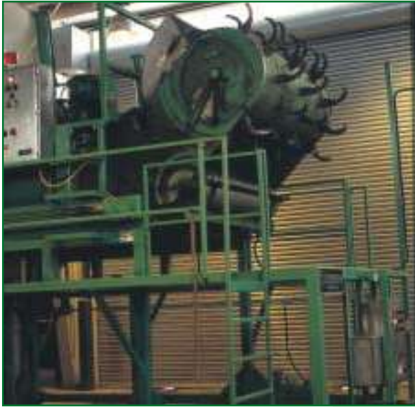
The agitator, pictured above, moves along the bays, slowly pushing the material forward as it mixes it. After 14 days in the bays, the food waste has broken down into compost.
