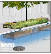
(ROWB). The Type 1 ROWB is 20' x 5' and can manage an average of 250 cubic feet or 1870 gallons of stormwater that flows along the curb during a storm event. You can see a ROWB in action here (
