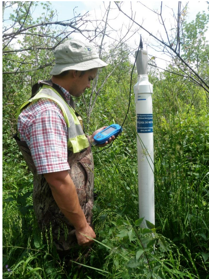
Figure 2.2. Data collection from an Ecotone™ monitoring well in the Schoharie basin (SMS).
