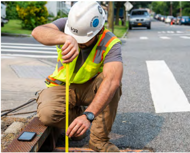
Measuring debris in catch basin for Loading Rate Study
