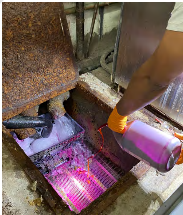
DEP conducts dye test to track down illicit discharge
