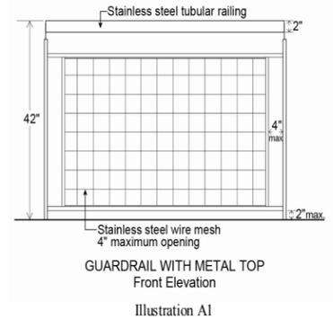
All guardrail components and hardware shall be in No. 316 Stainless Steel, passivated and bead blasted.
