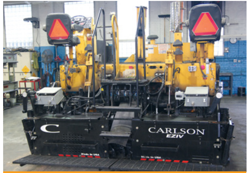
Paving machine with electric screed
