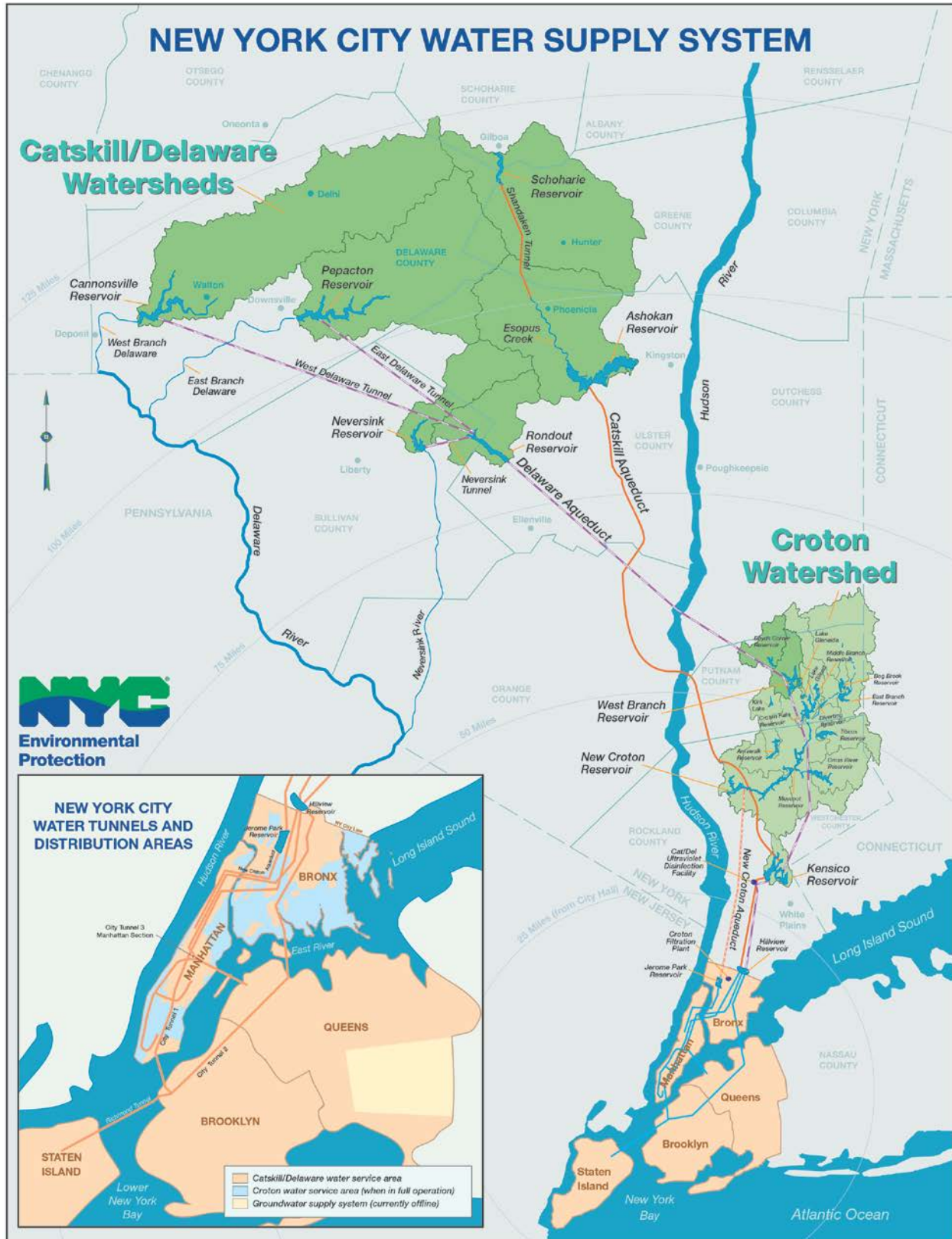
Figure 1-1: Water Supply System Map Source: DEP (2013)
