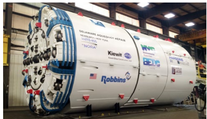
Custom-built tunnel boring machine being used for construction of the bypass tunnel
