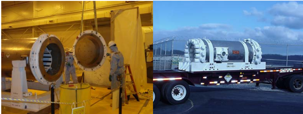
In February 2009, a Permit Was Issued for the Move of the Beam Plug of a High Flux Beam Reactor From Brookhaven National Laboratory. The Plug Was Loaded Into a Steel-Supported, Lead Lined Shipping Cask. Although the Metal is Radioactive, the Radiation Cannot be Dispersed. The Driver Was Federally Certified, Accompanied by Armed Escorts, and Only Traveled at Night.
