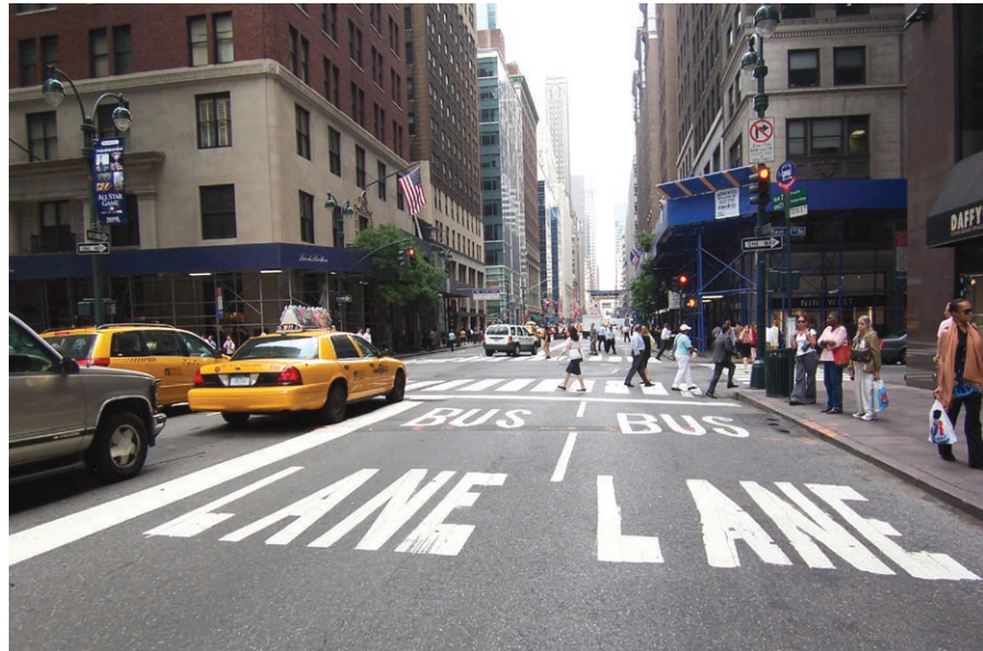
Curb-aligned double bus lane: Madison Avenue, Manhattan
