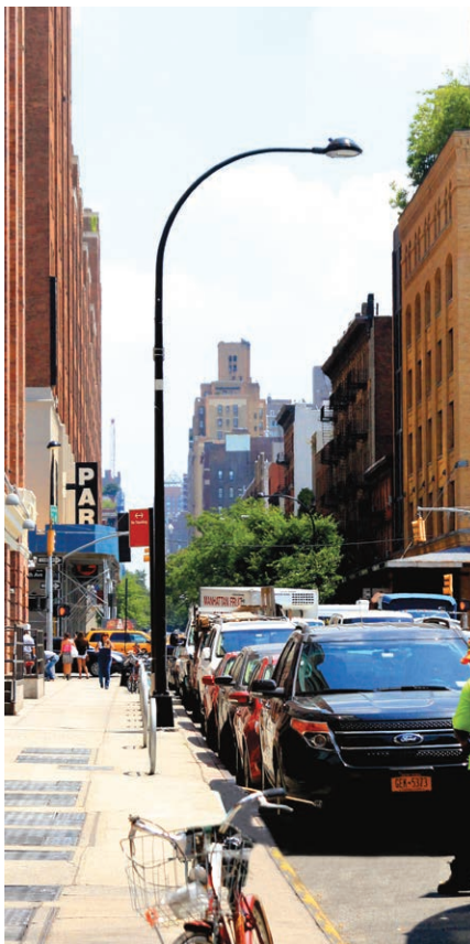
Standard poles can be painted black, brown, or green, and combined with the Helm or Stad luminaire. Such modifications are considered Standard but they typically require a maintenance agreement. West 15th Street, Manhattan.
