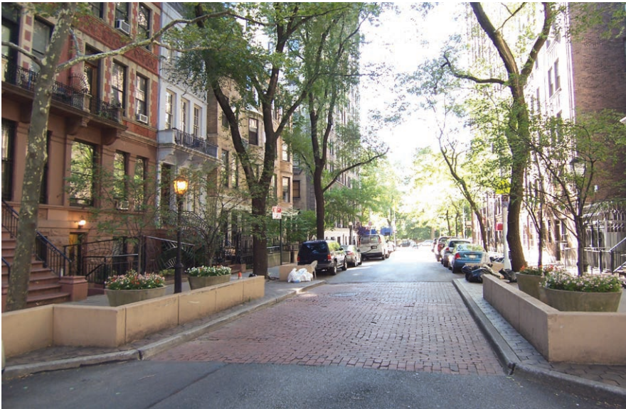
Mid-block narrowing: West 94th Street, Manhattan (Note: use of walls is not recommended by this manual)
