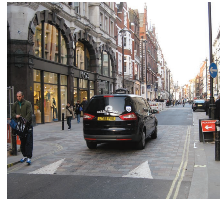
Raised crosswalk: London, United Kingdom (Note: for illustrative purposes only)
