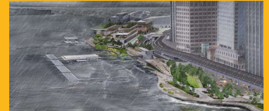
Illustration of how the buried floodwall and floodgates would protect Lower Manhattan during a coastal storm
